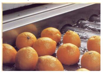
For complete coverage of an elongated fruit such as a lemon, the rolls not only rotate, but also oscillate horizontally in opposite directions causing the entire peel surface to be punctured, releasing the oil. The puncturing operation takes place beneath the surface of a shallow pool of water contained in the BOE to insure that there is no loss of oil to the atmosphere.
