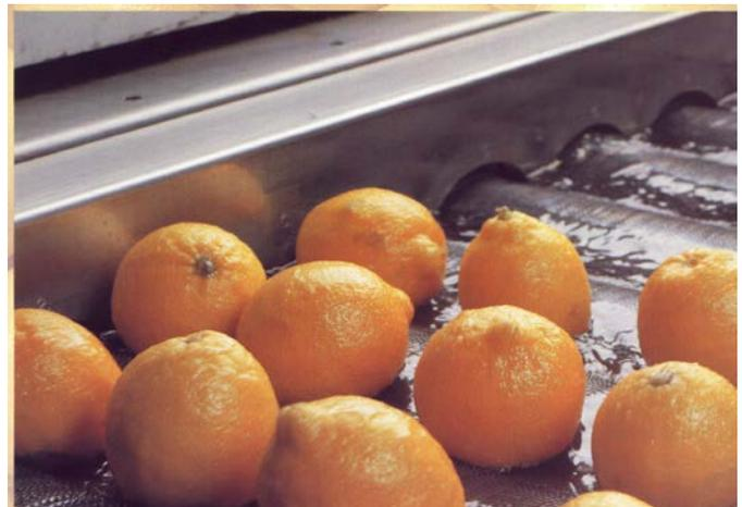
For complete coverage of an elongated fruit such as a lemon, the rolls not only rotate, but also oscillate horizontally in opposite directions causing the entire peel surface to be punctured, releasing the oil. The puncturing operation takes place beneath the surface of a shallow pool of water contained in the BOE to insure that there is no loss of oil to the atmosphere.
