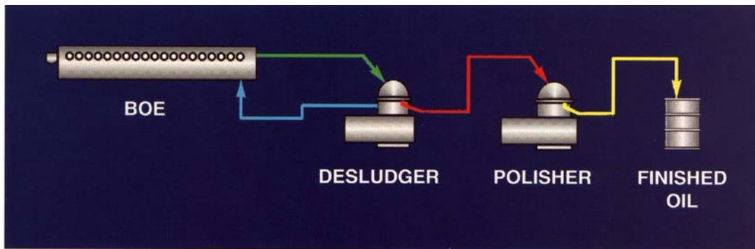
After leaving the BOE, the oil/water mixture passes through a fine screening operation in preparation for centrifugation. A first centrifuge produces a stream of rich oil. The water phase from this centrifuge is recycled back to the BOE to eliminate losses. Without costly freezing or enzyme treatment, the rich oil stream passes through a second centrifuge which continuously produces pure polished oil.
