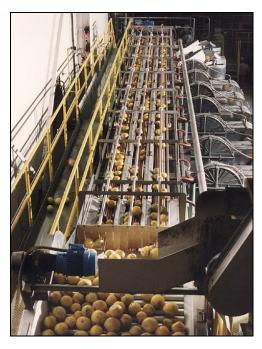
**APPLICATIONS:** The Model 5500 is readily adapted to accurately size and distribute various types of citrus fruit for processing. The volume of fruit to be processed and the types and numbers of extractors to be utilized determines the configuration of the sizer. The configuration of the sizer is the combination of the number of "runs" or sizing lanes and the length of the sizer or number of "bays".
